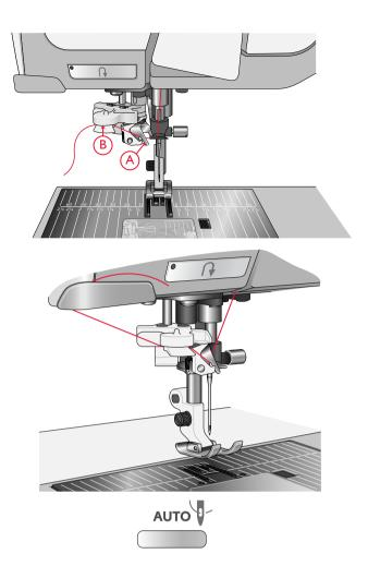
3. Touch the automatic needle threader button on the sewing head. The presser foot is automatically lowered during the threading sequence, and will rise again when threading is finished.
