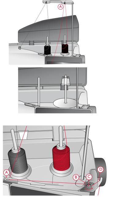
3. Place the bobbin on the bobbin spindle on the lower right side of the machine. The bobbin only fits on one way, with the logo facing out.
