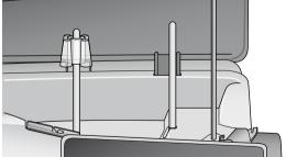
3. Hold the thread with two hands as illustrated. Floss the thread under the thread guide (A) from front to back. Pull thread back into and through threading slot (B).
