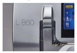
> Place the thread over the yellow thread take-up lever cover of the overlock needle and pull it down.
