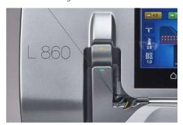
> Place the thread over the green thread take-up lever cover of the overlock needle and pull it down.
