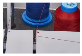
> Place the thread along the threading slot between the thread tension discs.
