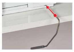
> To remove the Knee Lifter, pull the Knee Lifter out of the Knee Lifter Connection without swinging the Knee Lifter sideways.
