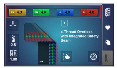
> The slider control of each thread tension can be adjusted between 1 and 9.
