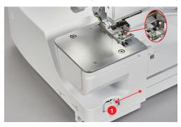
The knife, the stitch finger and the looper cover move in the corresponding direction as a result of the set knife position.
