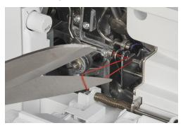
> Replace the looper thread on the thread stand with the desired special thread.
