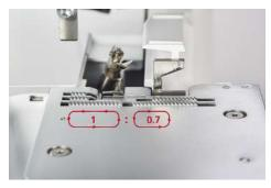
The front feed dog with the setting value 0.7 travels a shorter distance than the rear feed dog. This setting can also be used to deliberately stretch the material and to prevent seam puckering.
