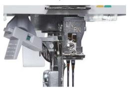
> Tighten the needle screws.
