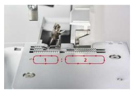
The front feed dog with the setting value 2 travels a longer distance than the rear feed dog at constant speed.
