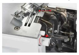
> To minimize the loops of the looper thread at the fabric edge, turn the mtc micro thread control in «-» direction during sewing.
