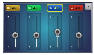
> Each individual thread tension can be adjusted between 1 and 9 using the fine adjustment keys «+/-». The alteration of the thread tension is visible on the screen.
