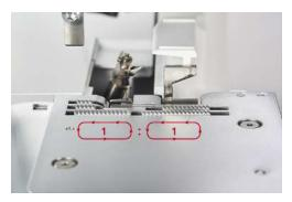
For default value 1, both feed dogs move by the same distance. The machine achieves an optimal sewing result for most applications regarding flat and even seams in the default value.
