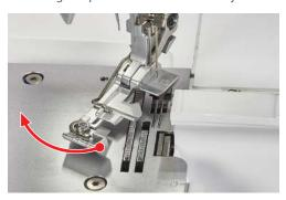
> To set the presser foot in the sewing position, lower the presser foot lifter or swing the presser foot sideways to the right.
