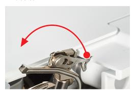
> Lightly press the upper looper converter back on the retaining bracket and hook the snap-in lug into the eye of the looper, making sure that the snap-in lug is completely engaged.
