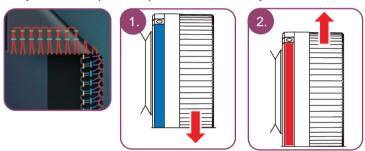
Needle thread (yellow) creates loops on bottom side of the fabric.
